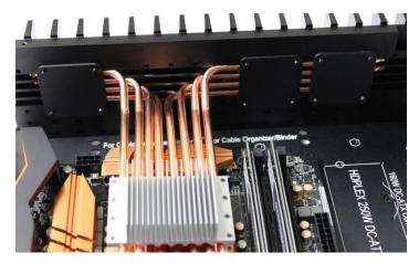
Apply a thin layer of thermal paste on each groove on the aluminum top plate and install the aluminum top plate using 8pcs **H-2**.
