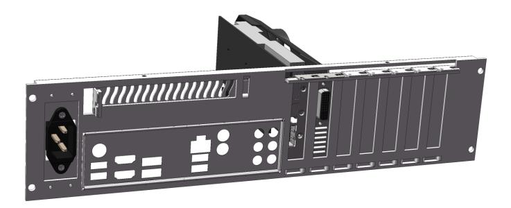
After everything is in place, you can lock the top of low-profile PCI-E expansion card using **A**.
