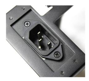
If you are using 7.4\*5.0mm self-lock connector, please install the DC Adapter Plate using 2pcs  $\triangle$  to the AC adapter plate.
