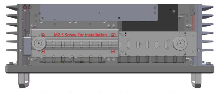
Four M2.5 mounting holes are circled in red. H5 bottom plate is made transparent for clear view. The four M3 holes in the center on the back of the 400W AC-DC adapter are not used for H5 mounting. HDPLEX 400W DC-ATX is front mounted using M3 screws. One 24PIN extension cable is included in the H5 package.
