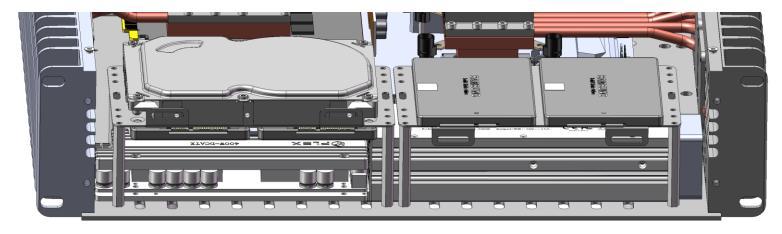
If you have a long video card or is using H5.TODD, you could double stack the second HDD rack with 3.5HDD on top of the first rack using 10mm copper stud.
