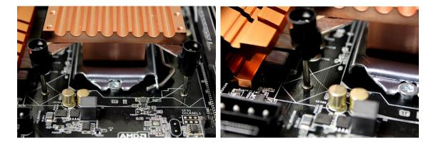
For the latest AM4 Ryzen socket, see below for correct rack installation position.
