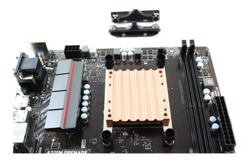
Apply thermal paste to the heatpipe groove on both side panels using the dumbbell shaped tool. Apply a thin layer of thermal paste to the copper plate groove using the dumbbell tool.
