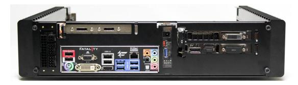
Lock the half height card using 1pcs A on the M3 thread hole
