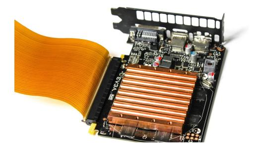
Install the video card to the H5 back plate. Slide the dual bracket tip inside and using 1pcs A firmly attach the video card bracket to H5 back plate.
