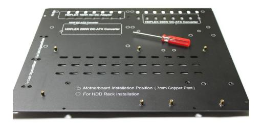
Install J to the back side of the H5 bottom plate, lock the copper stud M3 exposed thread.
