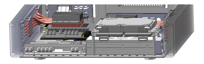
If you are using ITX motherboard, you can install the second HDD rack on the side position.
