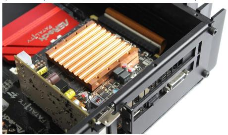
Apply thin layer of thermal paste to the side panel groove and install eight heatpipes following the below pattern.
