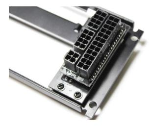
ATX Modular bridge board will conflict with H5 side heatsink panel if installed incorrectly. Below is the view from external side of the H5 backplate.
