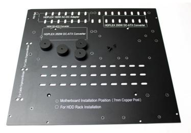
Install Hexagonal Copper Stud 7mm **E** to the bottom plate, matching your motherboard installation position
